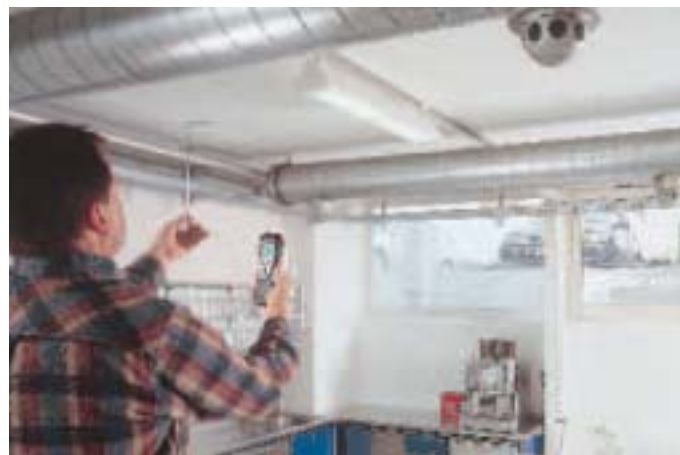
Measuring outlet air
