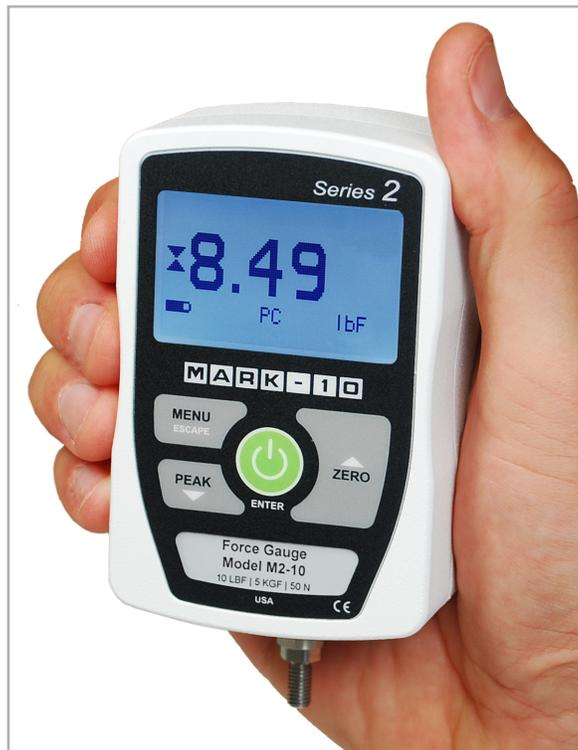
Series 2 digital force gauges are designed for basic tension and compression force testing applications up to 100 lbF (500 N). Peak tension and compression readings are reliably captured via the gauges'  $\pm 0.5\%$  accuracy and 500 Hz sampling rate. A backlit graphic LCD displays the current, peak tension, or peak compression reading.
