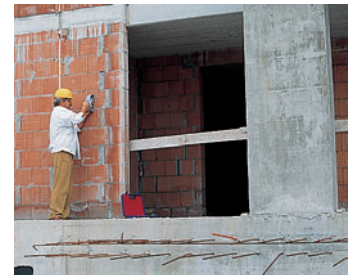
Type PM for quality control of mortar in masonry.
