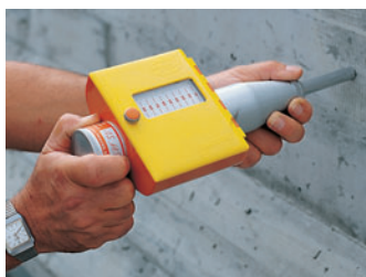
Perform test series of at least ten test impacts.
